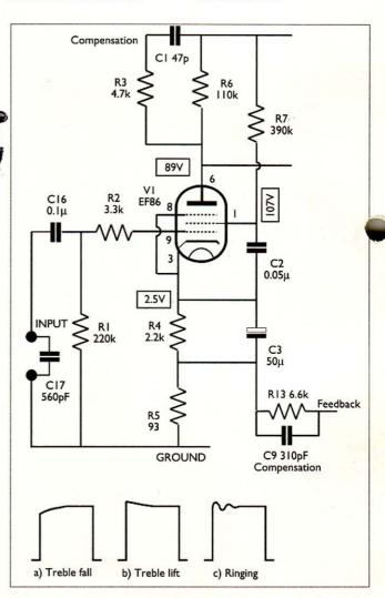
Feedback components have to be set depending on phase shift around the circuit. A scope can be used to view square wave performance which gives a useful guide.
