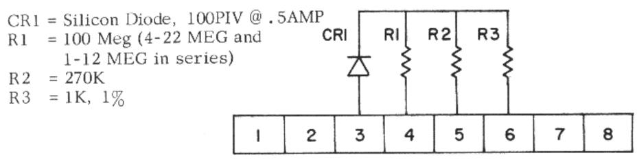
Figure 2. Cal Module Schematic
